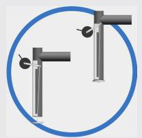
The automatic shut-off valve closes the outlet pipe when the maximum oil storage capacity is reached.
