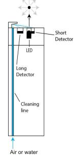
used to detect low and high concentrations of solids. The SoliSense® uses Pi's novel measurement technique that automatically takes readings at four different light levels and uses the gradient between the four readings to produce the sensor output. This configuration allows accurate and reliable measurements of suspended solids concentrations and turbidity to be made.
