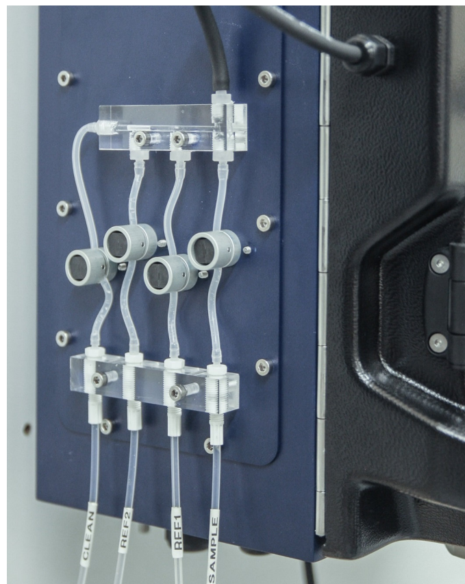
Image, right: pinch valves for standard solutions and sample handling, carefully isolated from the inside part of the EnviroLyzer® .
