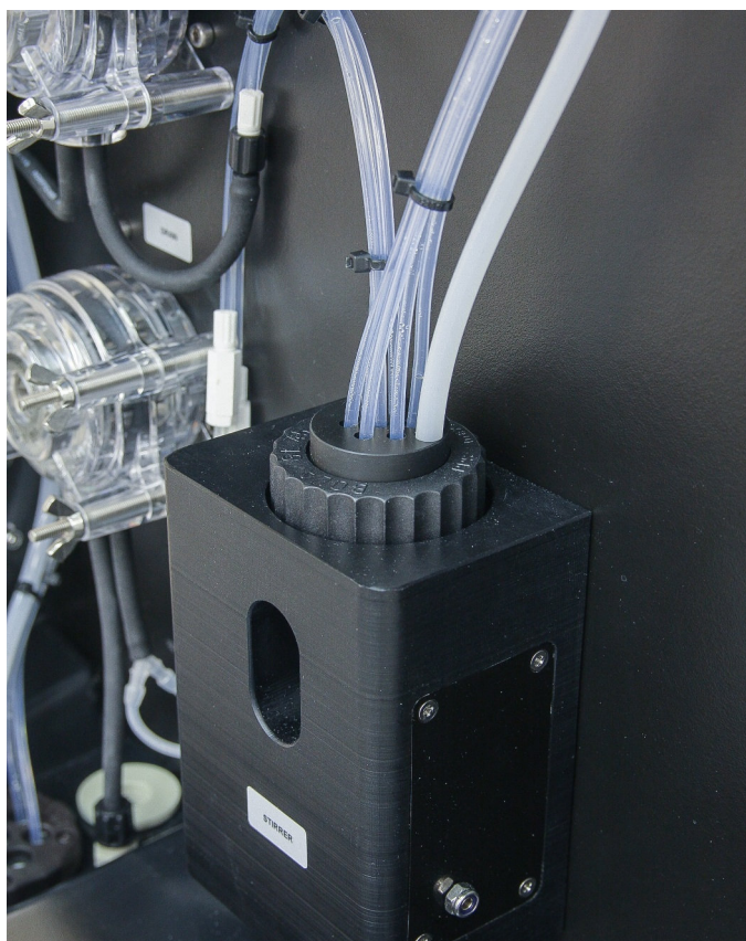
Image, left: photometer assembly with additional sample dilution.
