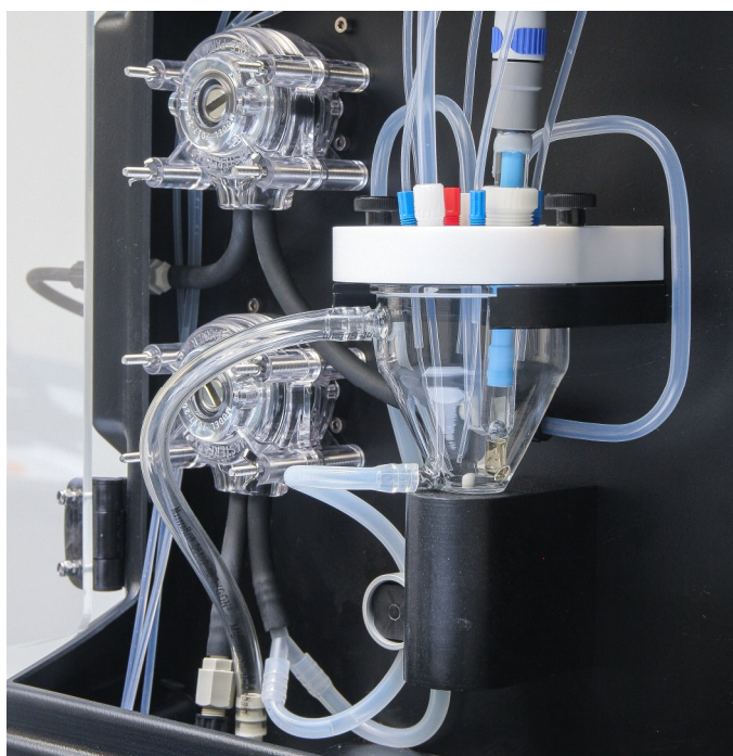
Image - inside the wet part of the AnaSense®: titration vessel with pH electrode, long-life peristaltic pumps for sample and drain.
